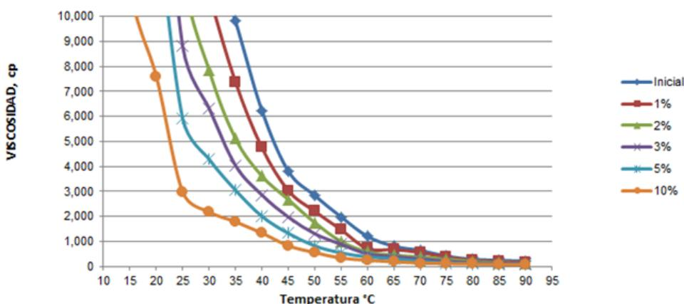
Figure 1.- Viscosity Reduction of a crude oil sample at different temperatures and dosages
